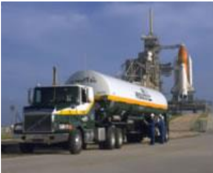
An Air Products truck delivering LH2 to the space shuttle Atlantis
